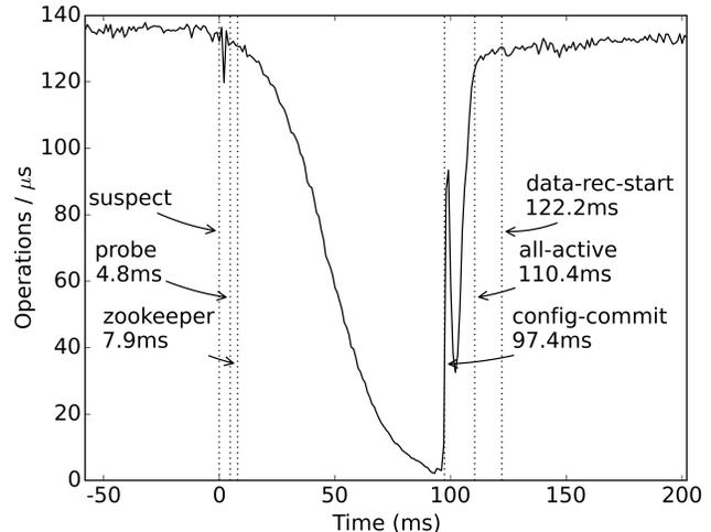
**Figure 11.** TATP performance timeline with CM failure
