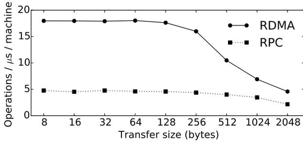
Figure 2. Per-machine RDMA and RPC read performance
