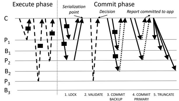
**Figure 4.** FaRM commit protocol with a coordinator  $C$ , primaries on  $P_1, P_2, P_3$ , and backups on  $B_1, B_2, B_3$ .  $P_1$  and  $P_2$  are read and written.  $P_3$  is only read. We use dashed lines for RDMA reads, solid ones for RDMA writes, dotted ones for hardware acks, and rectangles for object data.
